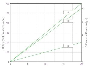
Flow (L / min) for liquid @ 20 °C and 1 cp per 10" module Recommended beer flow rates between 3 - 7L/min/10" module
