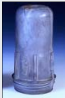
No corrosion with Alocrom treatment.
