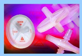
Lightweight and easy to use these filters have stepped hosebarb or NPT threaded connections offering a convenient and time saving method for connection. They eliminate the need for expensive reusable holders and ensure perfect sealing of the membrane every time. Their robust design allows for repeatably autoclaving where multiple batch use has been validated.
