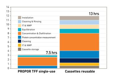
By switching to a fully disposable flow path, including the TFF filter, up to 5 hours of facility time can be saved during ultrafiltration applications compared to reusable cassettes. This is achieved by eliminating pre and post-use water permeability testing, pre-flushing, pre and post-use cleaning and cassette storage operations.
